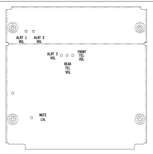
Figure 2-1. Access Hole Location (Top View)
